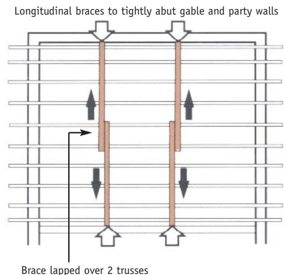
Fig. 4 Position of diagonal wind braces
