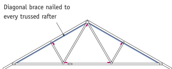
Fig. 5 Plan of rafter diagonal bracing on differing plan shapes
