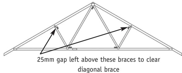
Fig. 3 The fixing of longitudinal braces
